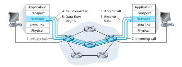
Figure 4.4 ♦ Virtual-circuit setup
