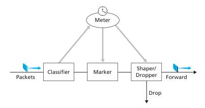
Figure 7.26 ♦ A simple Diffserv network example
