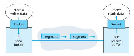
Figure 3.28 ♦ TCP send and receive buffers
