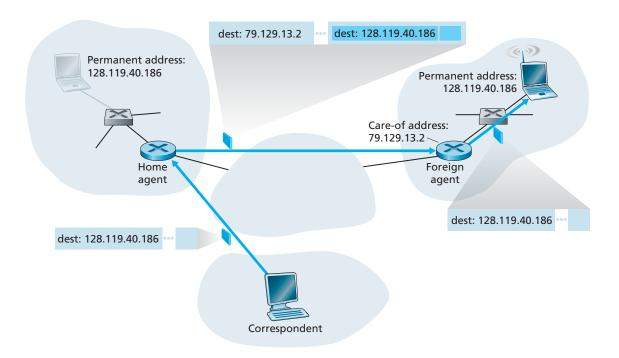
Figure 6.24 ◆ Encapsulation and decapsulation
