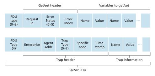
Figure 9.4 ♦ SNMP PDU format
