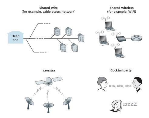
Figure 5.8 ♦ Various multiple access channels
