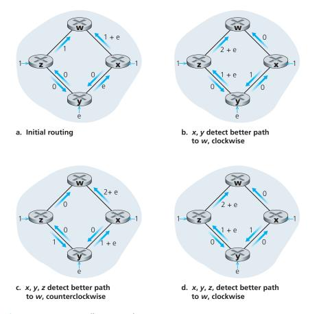
Figure 4.29 ♦ Oscillations with congestion-sensitive routing
