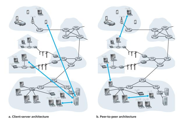
Figure 2.2 ♦ (a) Client-server architecture; (b) P2P architecture
