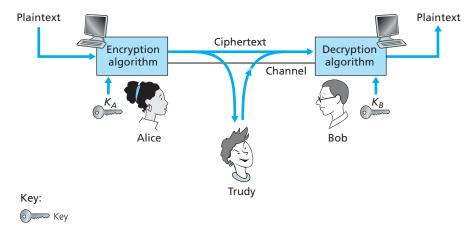
Figure 8.2 ◆ Cryptographic components
