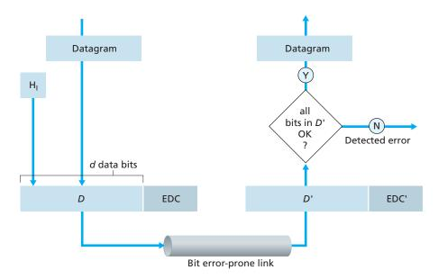
Figure 5.3 ◆ Error-detection and -correction scenario
