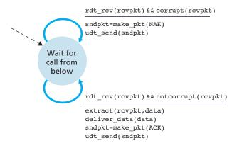
Figure 3.10 ♦ rdt2.0-A protocol for a channel with bit errors
