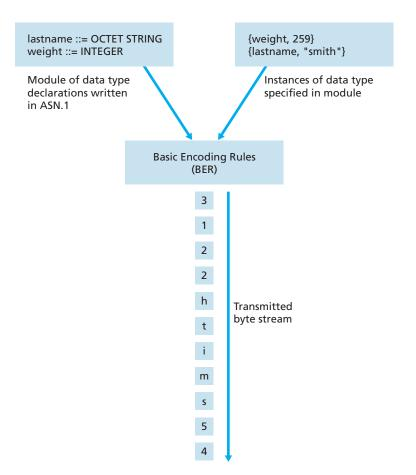
Figure 9.9 ♦ BER encoding example
