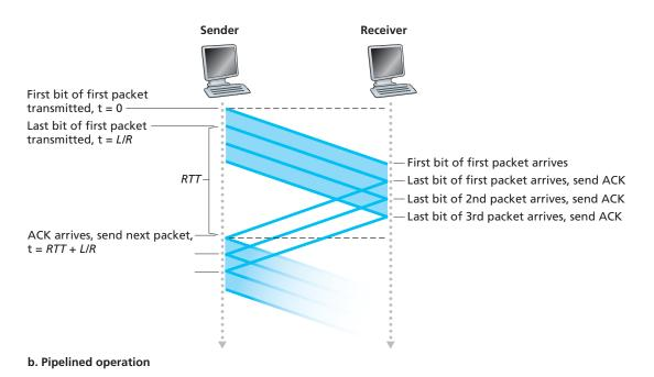
Figure 3.18 • Stop-and-wait and pipelined sending
