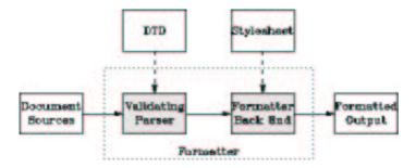
The part of the diagram inside the dotted box is your formatting software, or *toolchain*. Besides the obvious and visible input to the formatter (the document source) you'll need to keep the two hidden inputs of the formatter (DTD and stylesheet) in mind to understand what follows.
