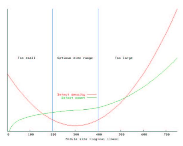
This unexpectedly high incidence of bugs at small module sizes is robust across a wide variety of systems implemented in different languages. Hatton has proposed a model relating this nonlinearity to the chunk size of human short-term memory. <sup>[14]</sup>
