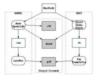
Figure 16.4. XML and SGML toolchains compared
