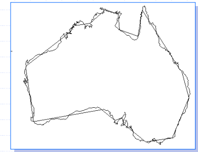
Min-# solution as shortest path in the digraph G_\varepsilon(P) .
